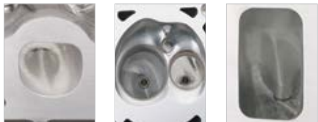
B Close-up shots of the COPO-specific CNC porting applied to an LS7 head
