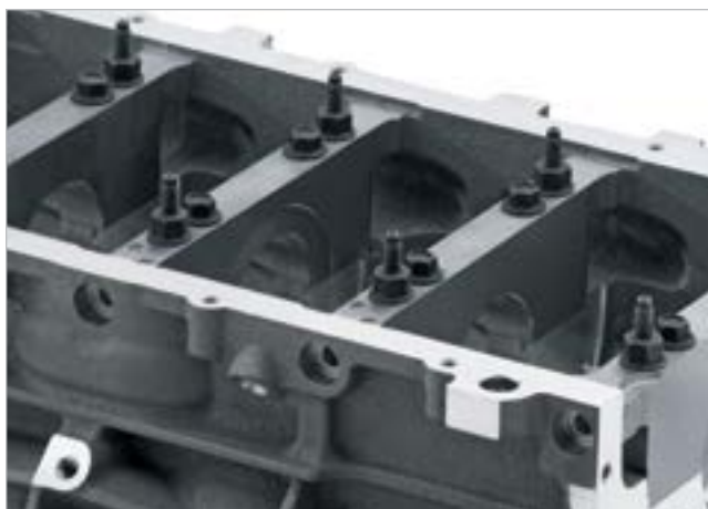
LS1/LS6 5.7L Block – Aluminum Block with 6-Bolt Main Caps A
